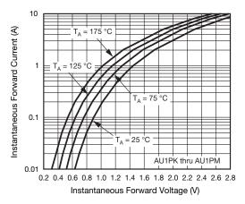
Fig. 5 - Typical Instantaneous Forward Characteristics
