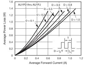
Fig. 2 - Forward Power Loss Characteristics
