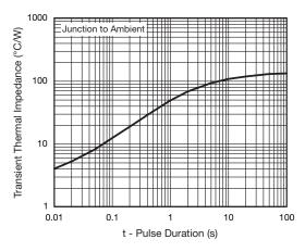
Fig. 9 - Typical Transient Thermal Impedance
