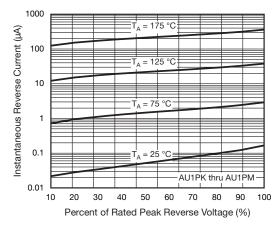
Fig. 7 - Typical Reverse Characteristics
