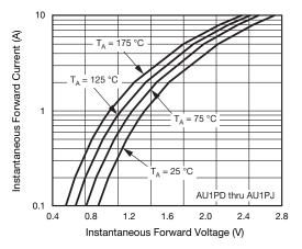
Fig. 4 - Typical Instantaneous Forward Characteristics
