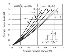
Fig. 3 - Forward Power Loss Characteristics
