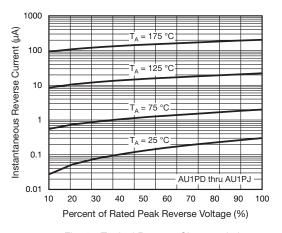
Fig. 6 - Typical Reverse Characteristics
