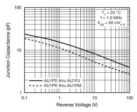
Fig. 8 - Typical Junction Capacitance
